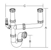
Flexible installation with full width and height adjustment
